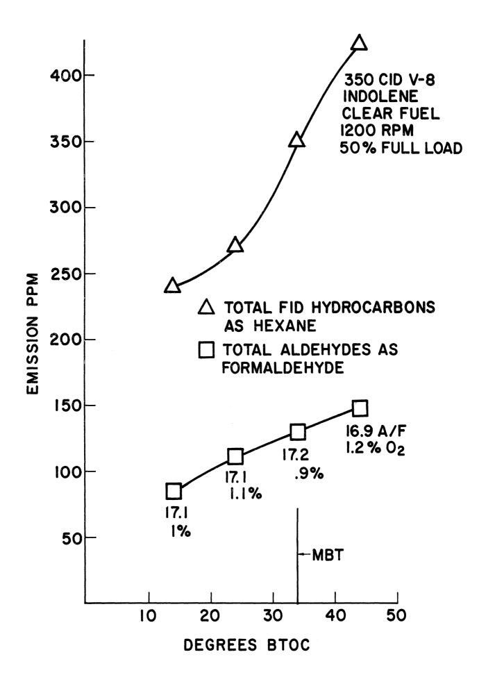
air-fuel ratio is indicated on the curve. More data will be taken on the standard engine.
