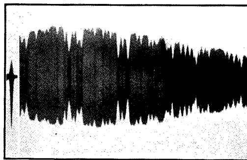
FIG. 4. The far infra-red spectrum of D_2O between 31\mu and 38\mu .
