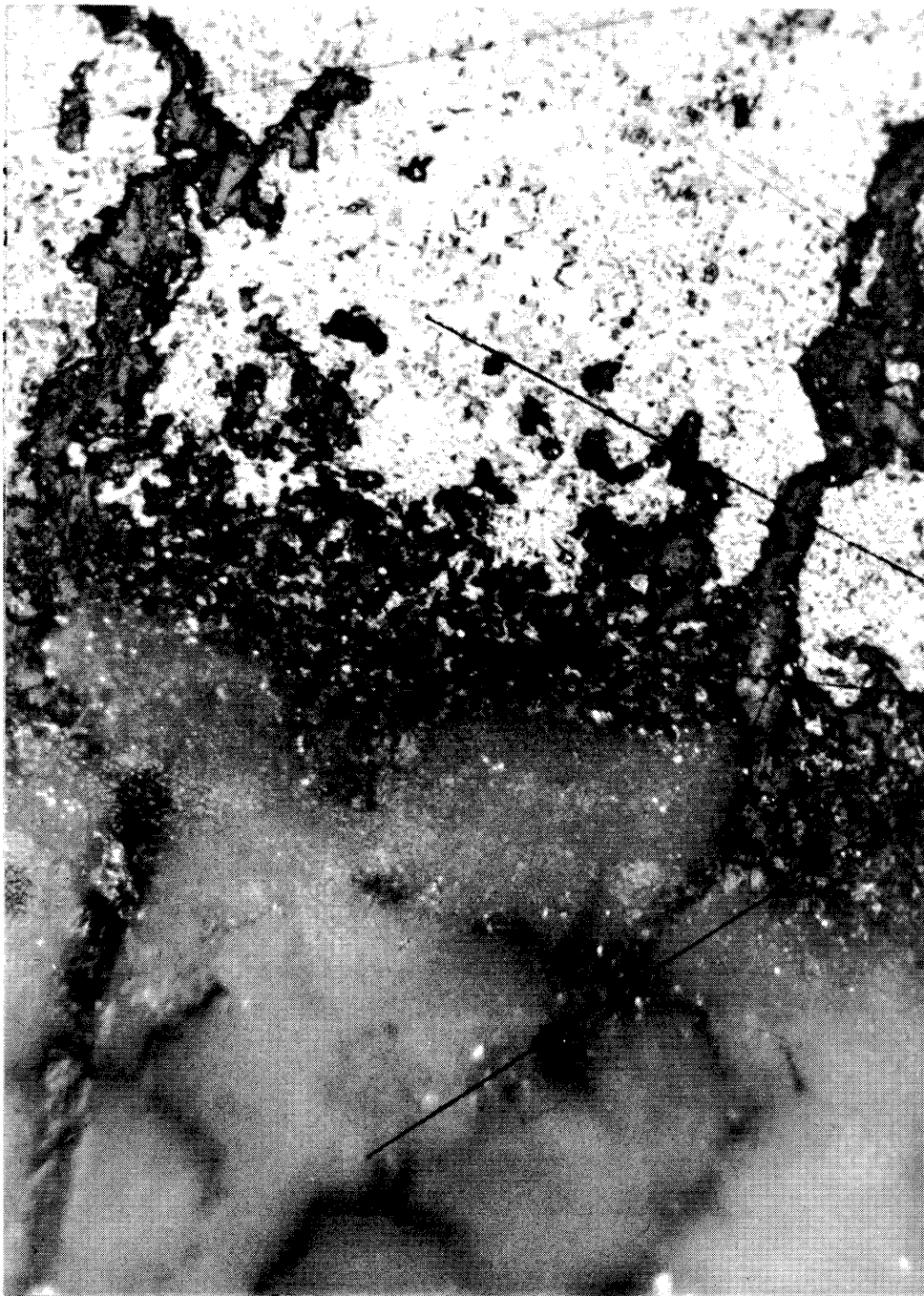
Figure 14: Photomicrograph at 50X of Lime Sample from Fine-Grained Stone Reacted with 20\text{SiO}_2 - 80\text{FeO} Slag at 1470^\circ\text{C} (Enlarged 2 times for reproduction)
