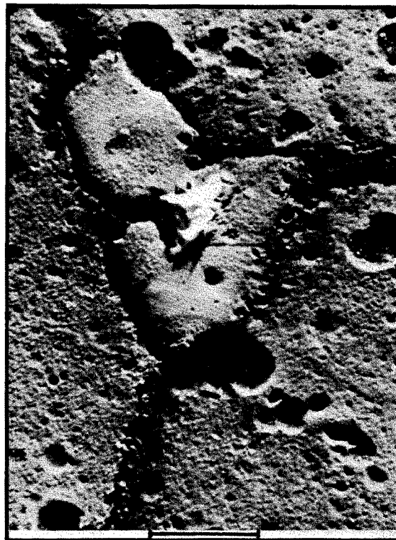
FIG. 11. A gold-shadowed collodion replica of a piece of magnesium etched with salt water.
