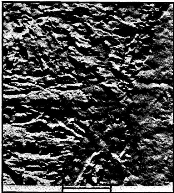
FIG. 9. A gold-shadowed collodion replica of an etched steel surface.
