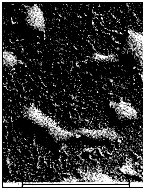
FIG. 17. A gold replica of polystyrene molecular fragments on a glass surface.
