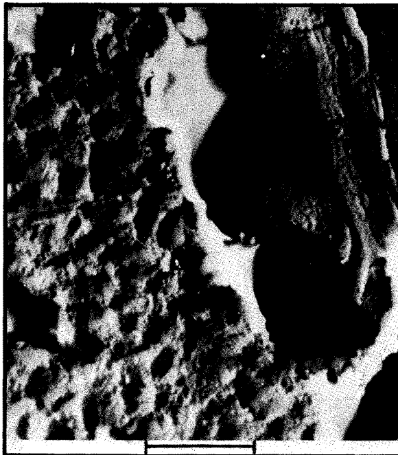
FIG. 10. A gold-shadowed collodion replica of an etched surface of 60-40 brass.
