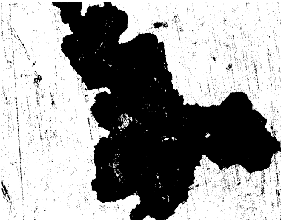
Fig. 5. Removal of Chromium Plate. Area outlined by original cracks in plate, sleeve 2, 100X.
