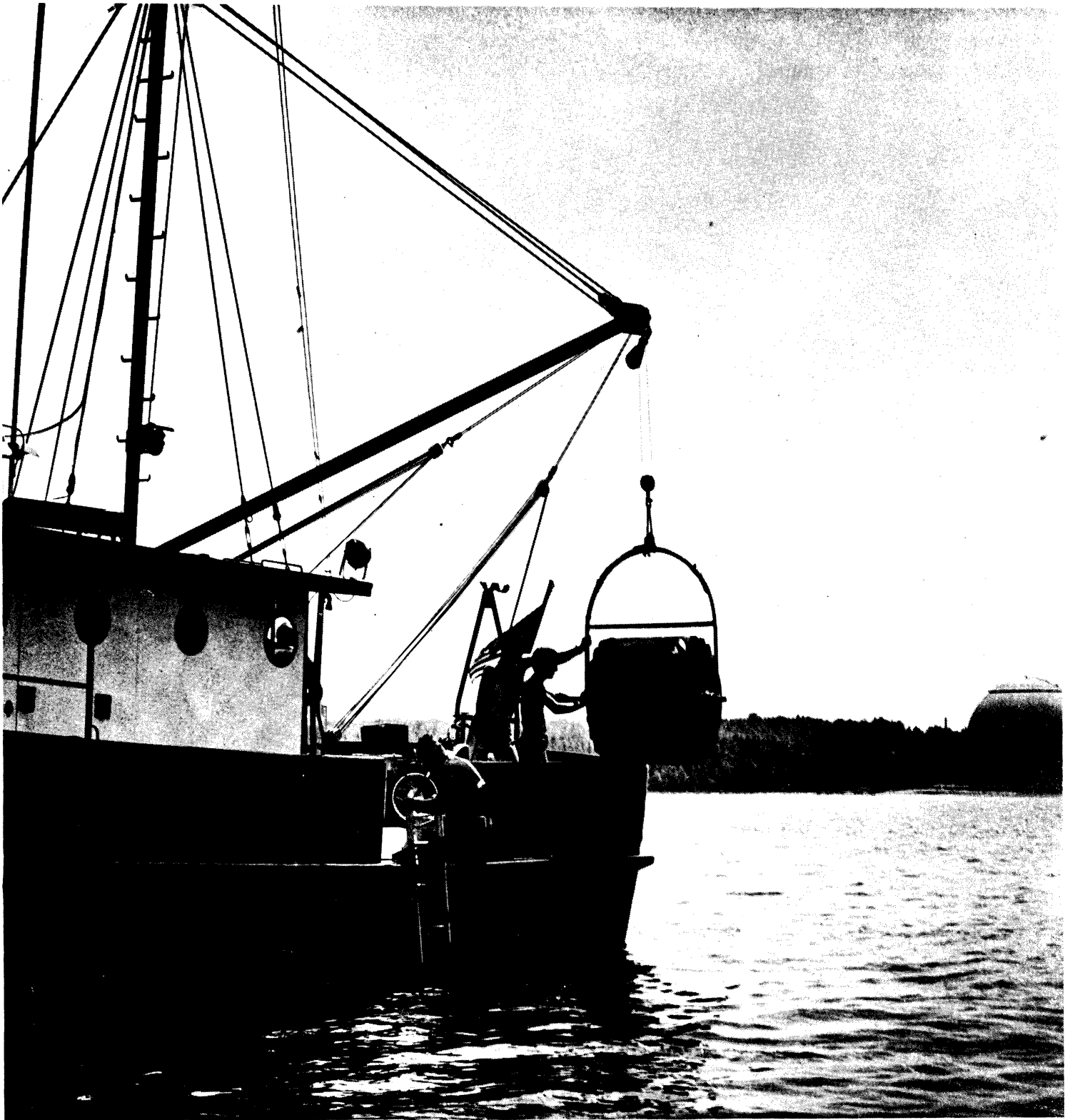
FIGURE 6. UNDERWATER GAMMA RADIATION DETECTION SYSTEM BEING PREPARED FOR FIELD WORK NEAR BIG ROCK NUCLEAR POWER PLANT.
