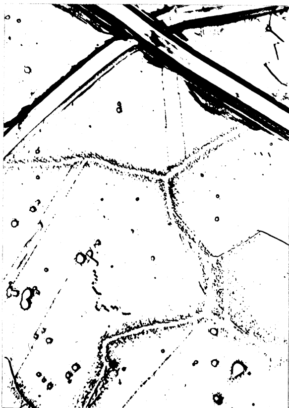
Optical photomicrograph X1000 Electrolytically etched in 10% chromic acid
