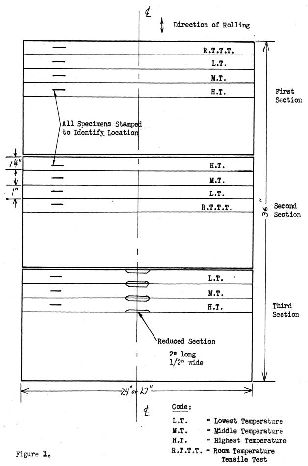
SKETCH INDICATING PROPOSED SAMPLING PROCEDURE OF SHEET MATERIALS WITH THE 36-INCH DIMENSION PARALLEL TO DIRECTION OF ROLLING.
