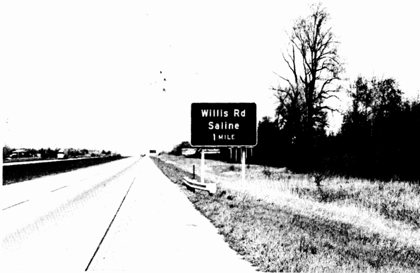
Sign 16. "Willis Rd.," Background - 17 \text{ cp/ft-c/ft}^2 , Legend - 86.5 \text{ cp/ft-c/ft}^2 , 5.1:1, 16" - 12", V = 13, H = 20.
