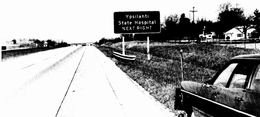
Sign 17. "Ypsilanti," Background - 6.2 \text{ cp/ft-c/ft}^2 , Legend - 92.7 \text{ cp/ft-c/ft}^2 , 15:1, 13.3" - 10", V = 11.5, H = 19.
