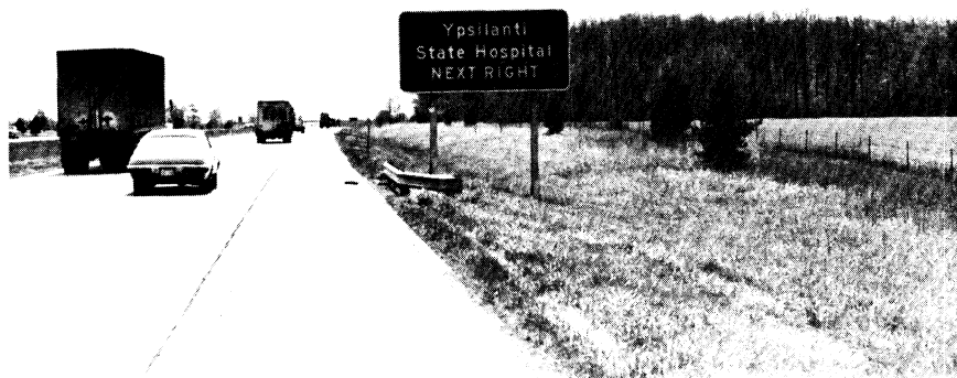
Sign 7. "Ypsilanti," Background - 20.1 \text{ cp/ft-c/ft}^2 , Legend - 77.3 \text{ cp/ft-c/ft}^2 , 3.8:1, 13.3" - 10," V = 12 , H = 21 .
