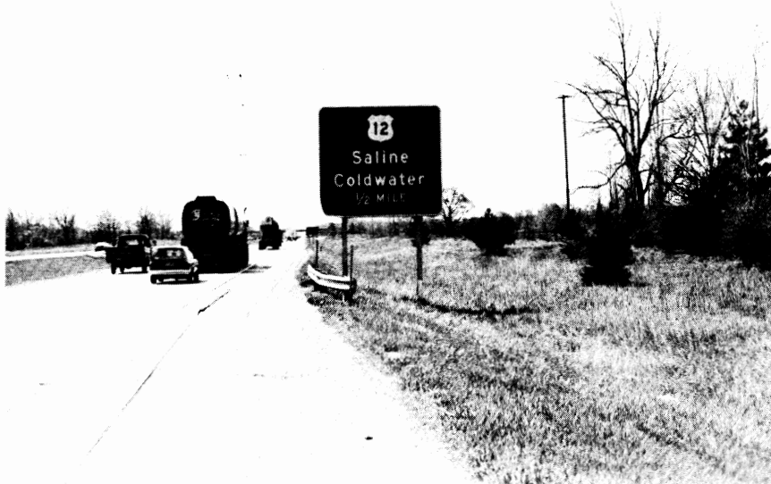
Sign 4. "Saline," Background - 18.9 \text{ cp/ft-c/ft}^2 , Legend - 74.2 \text{ cp/ft-c/ft}^2 , 3.9:1, 16" - 12," V = 12.5, H = 20.
