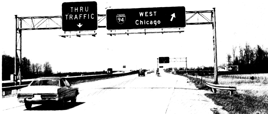
Sign 23. "West Chicago," Illuminated sign, Background - 2 ft-L, Legend 14 ft-L, 7:1, 16" - 12", V = 20.
