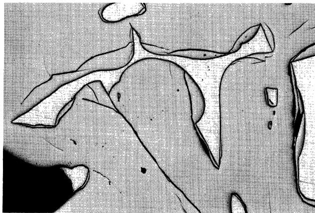
b) Equilibrated at 600°C for 72 hours. True dihedral angle: 64°.
