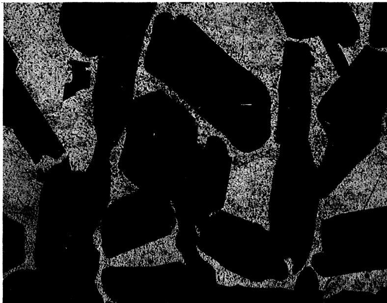
a) Aluminum-indium-rich liquid. True dihedral angle: 67^\circ .
