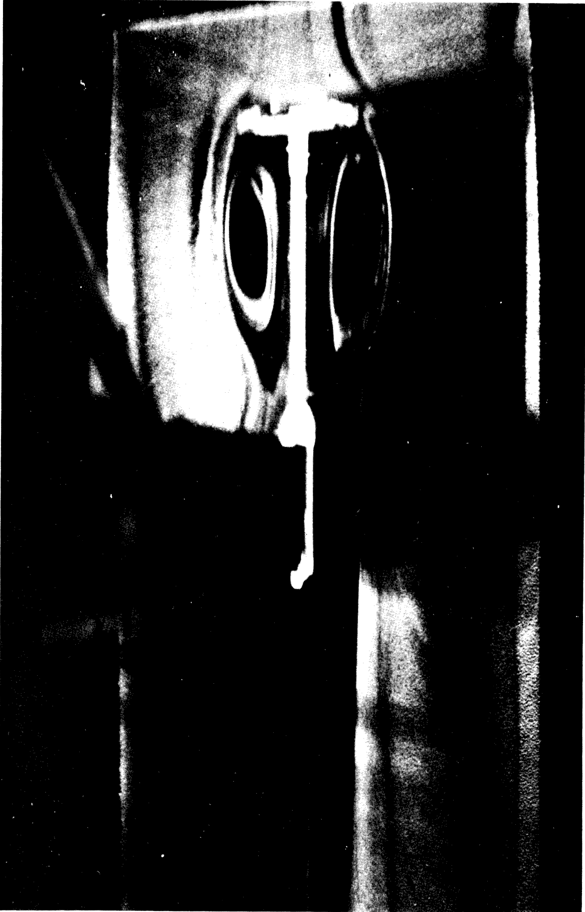
Figure 41. Photograph of steady flow about a sting-mounted disk at Re_d = 157 .
