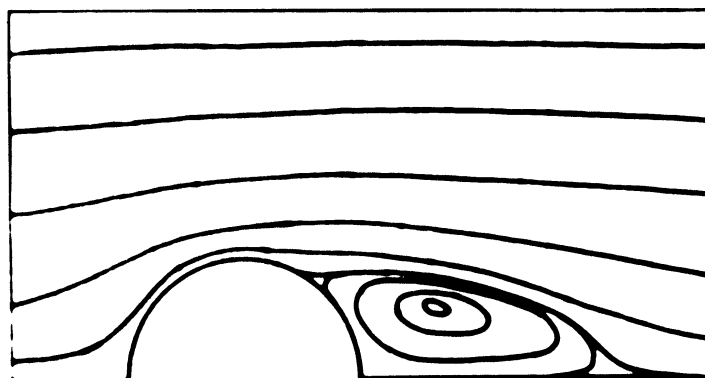
Figure 3. Sphere streamlines for Re_d \approx 100 .
