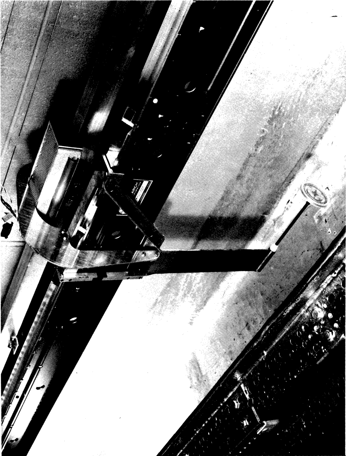
Figure 11. Photograph of carriage with disk mounted on balance.
