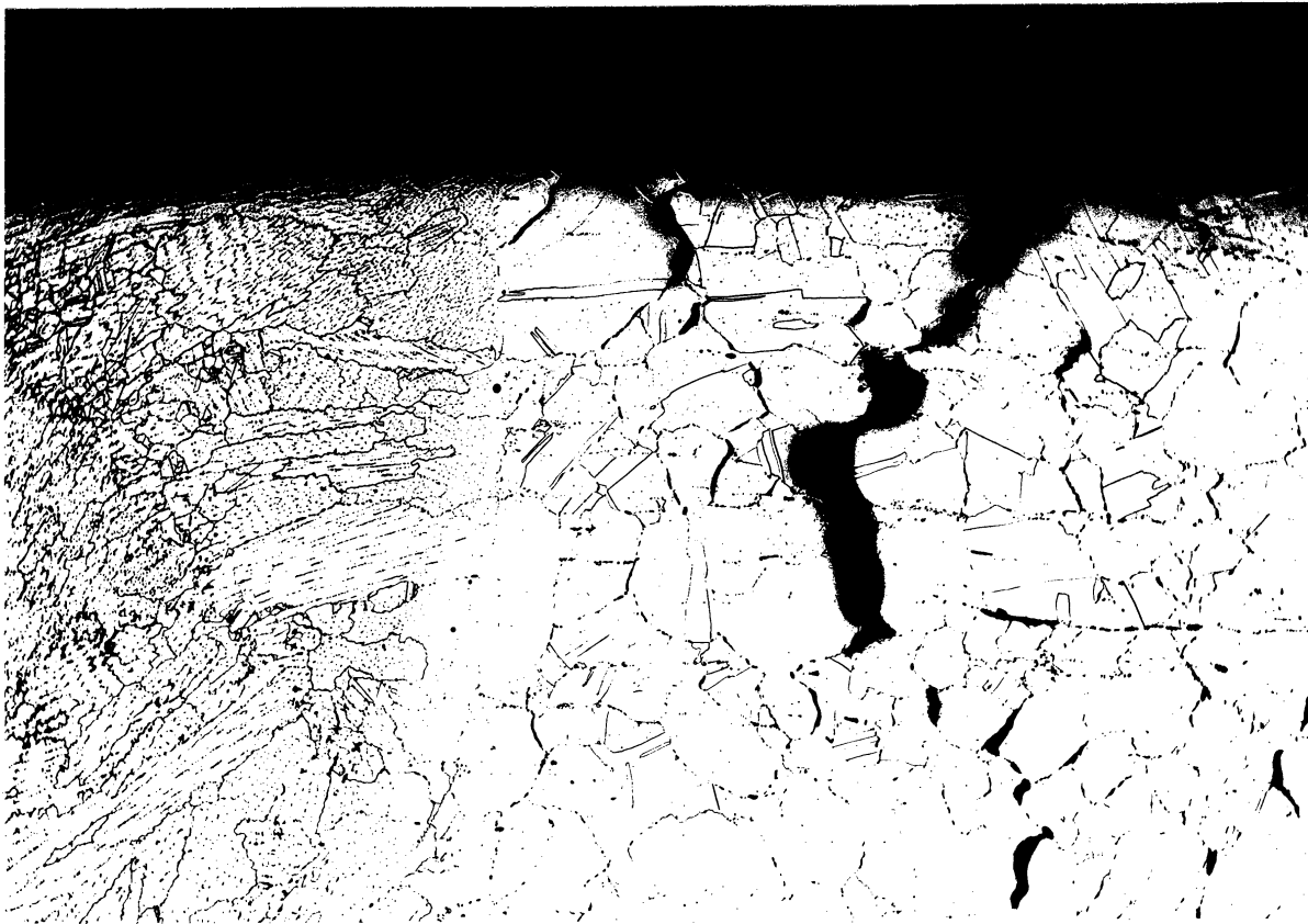
b. Cracks in Base Metal Near Weld Bond Line of Fractured Stress-Rupture Specimen - X100D
