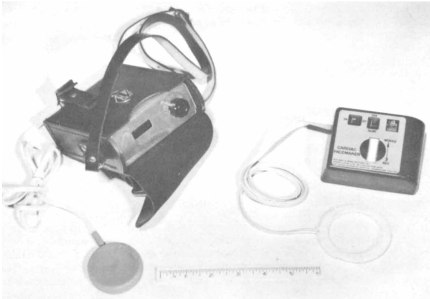
FIGURE 7. Left: Pacemaker and external coil used from late 1960 until mid 1963. Right: New pacemaker and external coil.
