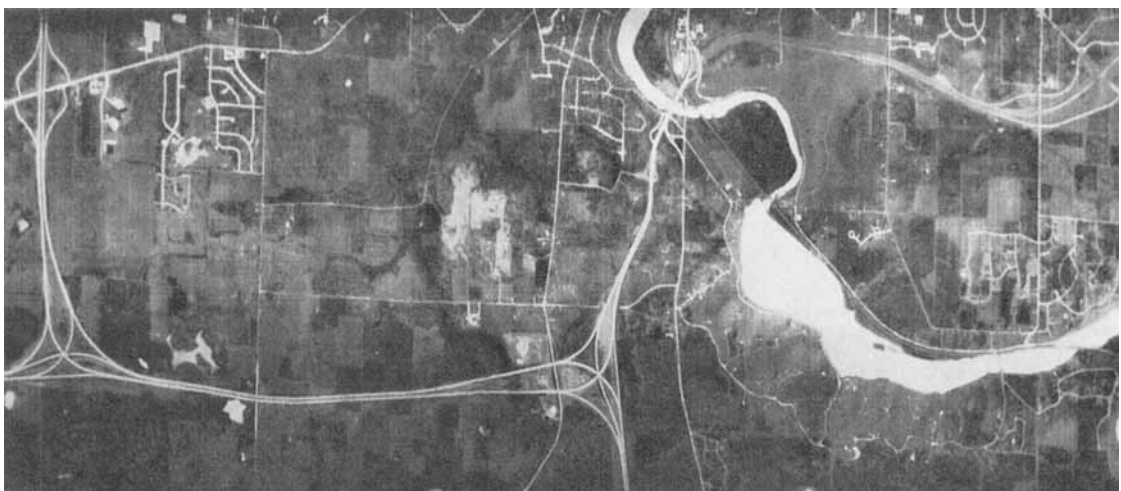
FIG. 2. Infrared Imagery in the 4.5 to 5.5 Micron Band of the Area Near Ann Arbor, Michigan, Shown in Figure 1. This imagery was obtained late on the night of July 20, 1965, from an altitude of approximately 10,000 feet. (Courtesy of the U.S. Forest Service.)
