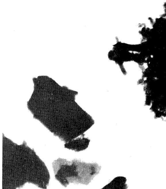
Figure 25. Electron Micrographs of Carbon Particles Deposited During Synthesis at a Magnification of 20,000 Diameters.
