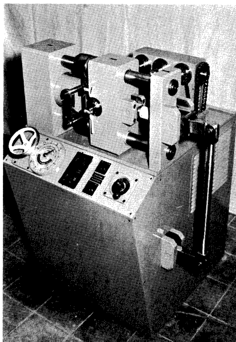
FIGURE 9. DETERMINATION OF SURFACE FINISHES OBTAINABLE BY COLD ROLLING. Present tests concern dimensional accuracy of cylindrical parts which have been rough turned. Brunswick.
