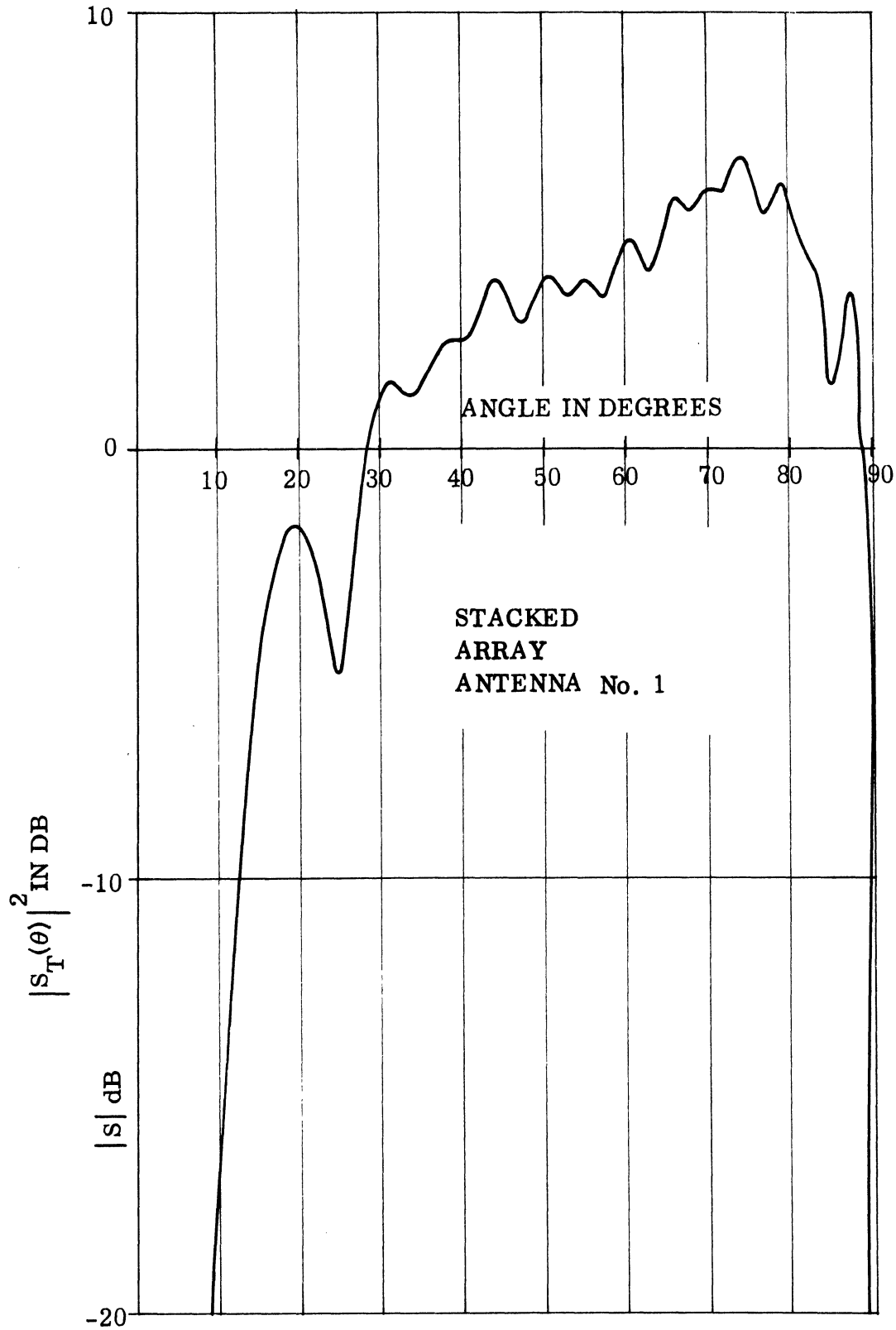
Fig. 3-3c: Theoretical elevation plane pattern of the optimum stacked array antenna. Z_0 = 50' .
