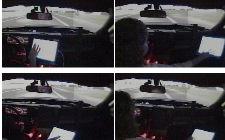
Figure 3.1. A subject is shown performing the in-vehicle task with the touch screen monitor in each of the four locations. Counterclockwise from top-left, the positions are near high, near low, far low, and far high.
