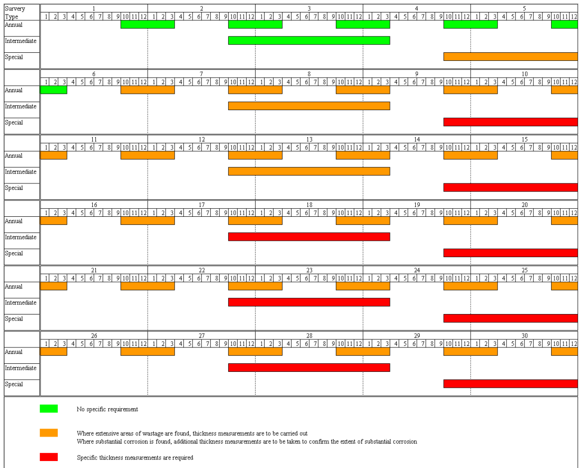
Figure 1.4 Typical thirty-year gauging survey plan for oil tankers
