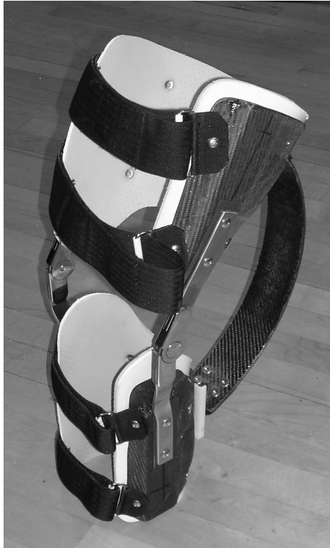
Figure 2.4 First generation prototype utilizing pre-impregnated carbon composite for the brace and leaf spring. Total brace weight—1.6 kg (3.5 lbs). Net rotational stiffness—2.8 N·m/deg (2.0 ft·lbf/deg).
