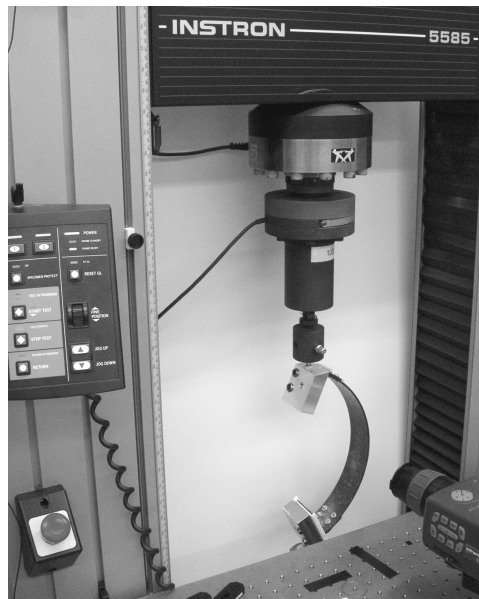
Figure 2.8 Quasi-static (1 in/min) compression testing was used to refine and validate the analytical model. Testing was performed on an Instron Model 5585 with a 4.45 kn (1000 lb) load cell.
