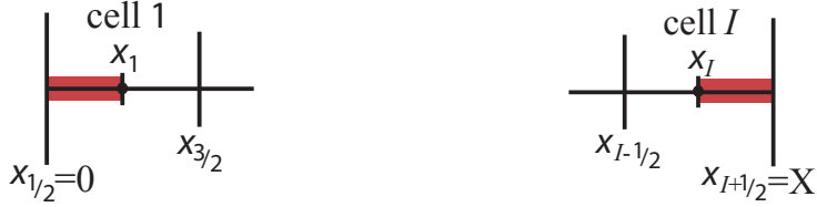
Figure 2.4 The Region of Integration for the Left ( left ) and Right ( right ) Boundaries
