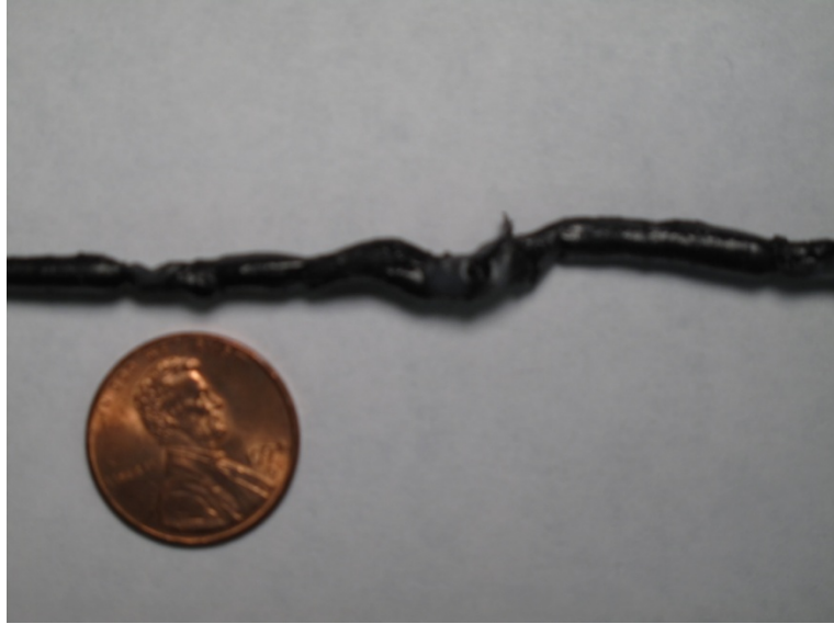
Fig. 7.22: Co 2 Z-LDPE/HDPE fibers after coextrusion to show a distorted shape due to the unsteady movement of materials inside the die
