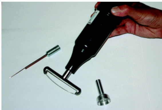
Figure 2.4. Handheld corona treater (model BD20-AC) with detachable electrodes. Electro-Technic Products, Inc.
