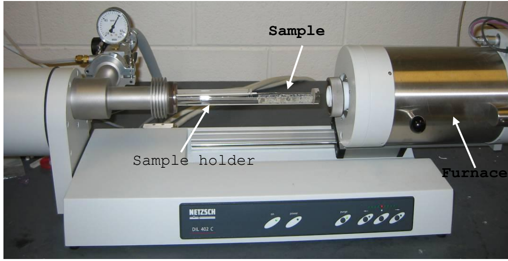
Figure 3- 6 Dilatometer for LTD test
