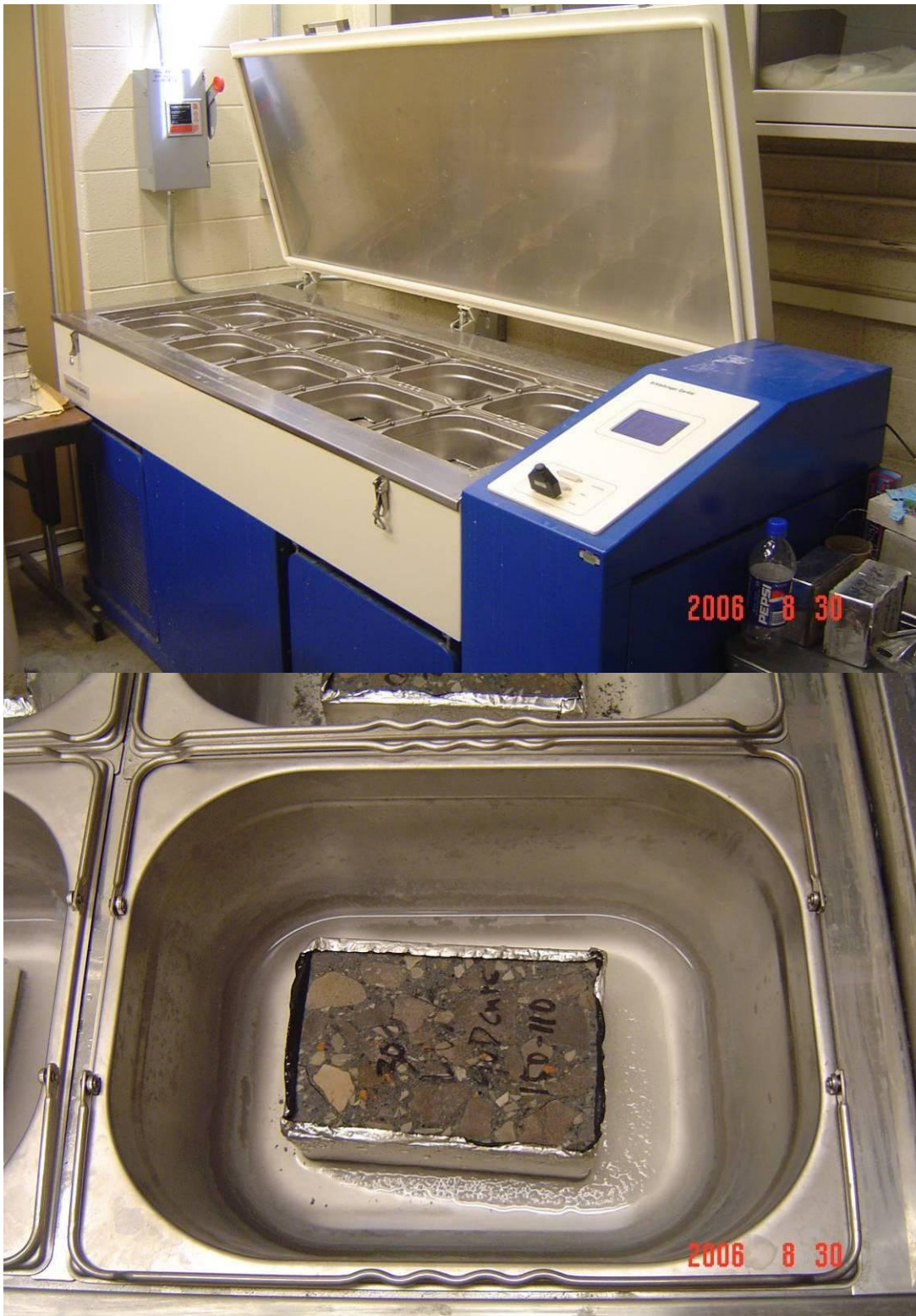
Figure 3- 3 Temperature controlled chest & Test container
