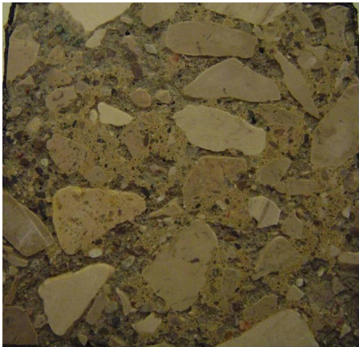
Figure 7- 45 OPC-II (after 10 F-T cycles in 3% NaCl solution)
