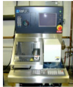
b) Computer-controlled dicing saw used for cutting wafers.
