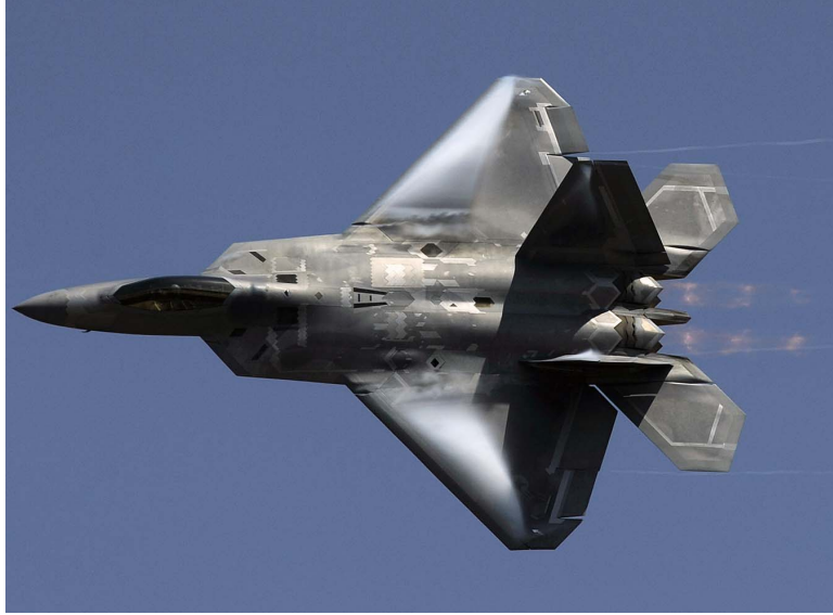
Figure 3.3: Steady flight (vehicle trim), is achieved by extending the flaps a small angle for the F-22 Raptor, a supersonic fighter aircraft [81].
