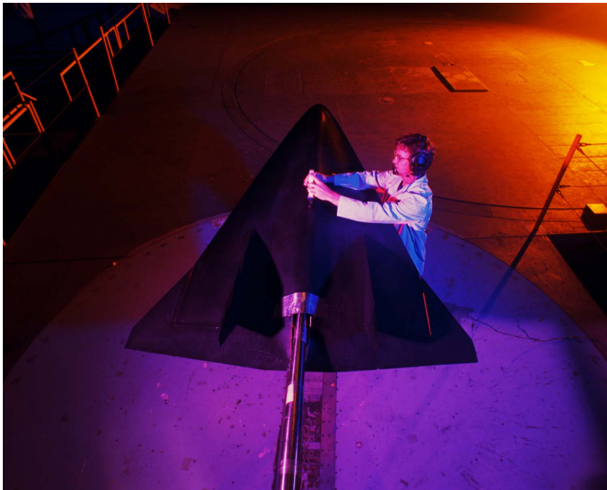
Figure 1.2: Mach 5.5 wave rider being prepared for a full scale wind tunnel test. (Great Images in NASA library, http://grin.hq.nasa.gov , image: GPN-2000-001927)
