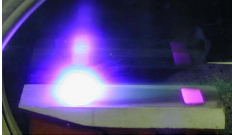
Figure 6.1: Glow discharge on a flat plate in Mach 5.2 air flow with a potential difference of 2800V (50 mA). Image from Kimmel et al. [28].
