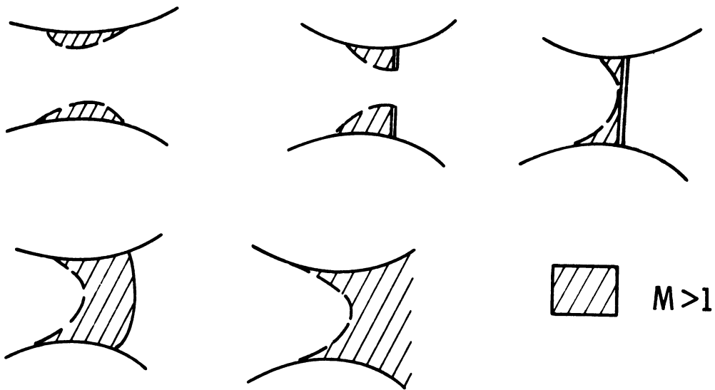
Figure 2. Transition from Taylor to Meyer type of nozzle flow as postulated by Emmons (1946).
