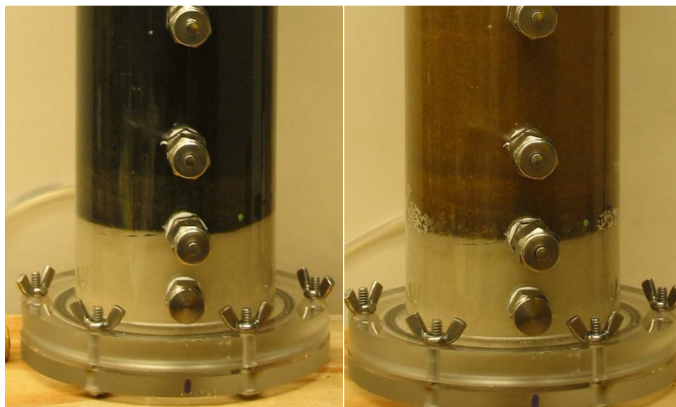
Figure 6.5: FeS-O 2 column changes in color: initially (left), and at 230 PV (right).
