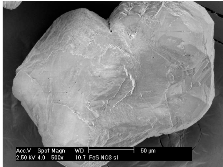
Figure 6.12: Grain of FeS-coated sand from the influent section of the FeS-NO 3 column.
