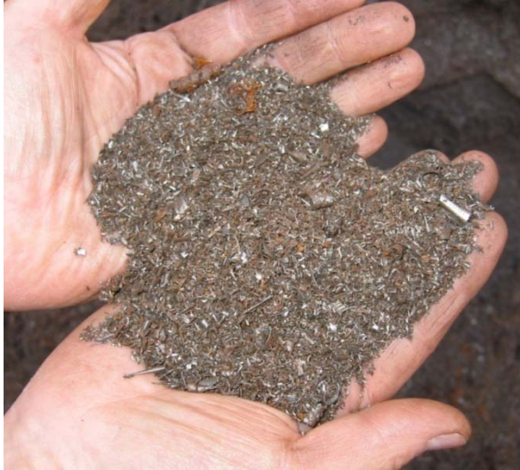
Figure 2.2: Waste iron millings, before further milling to create ZVI.
