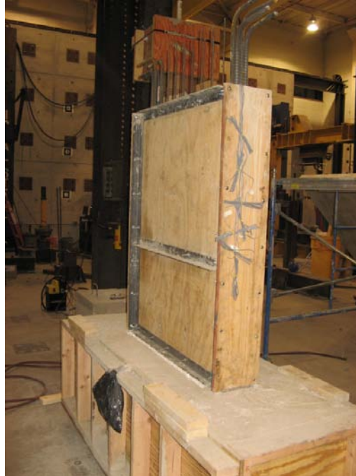
Fig. 3-24 Wall Ready for Casting (Specimen S10)
