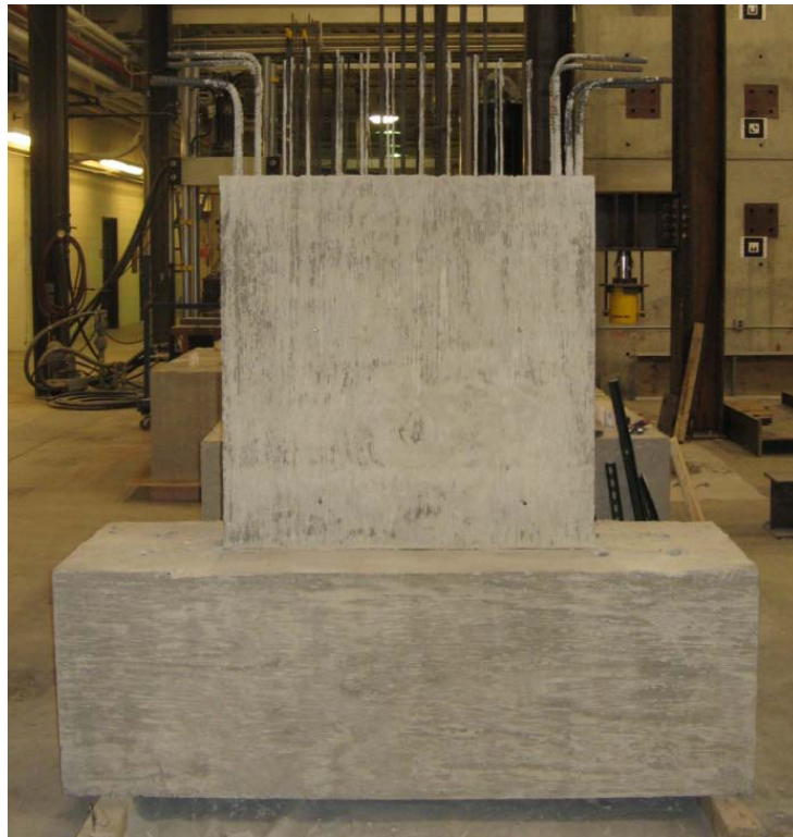
Fig. 3-25 Bottom Beam and Wall after Removal of Formwork (Specimen S4)
