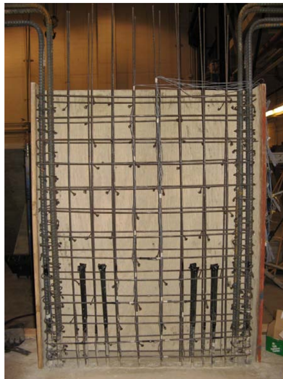
Fig. 3-23 Elevation View of Wall Reinforcement Layout (Specimen S10)
