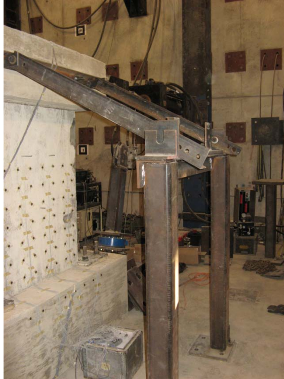
Fig. 3-33 Lateral Bracing Scheme (Specimen S10)
