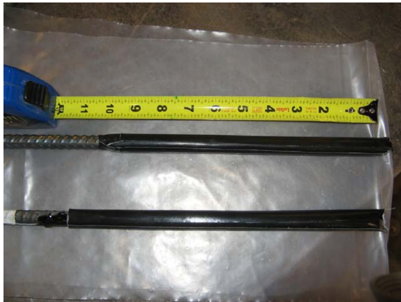
Fig. 3-8 Sleeves in Dowel Reinforcement (Specimen S10)
