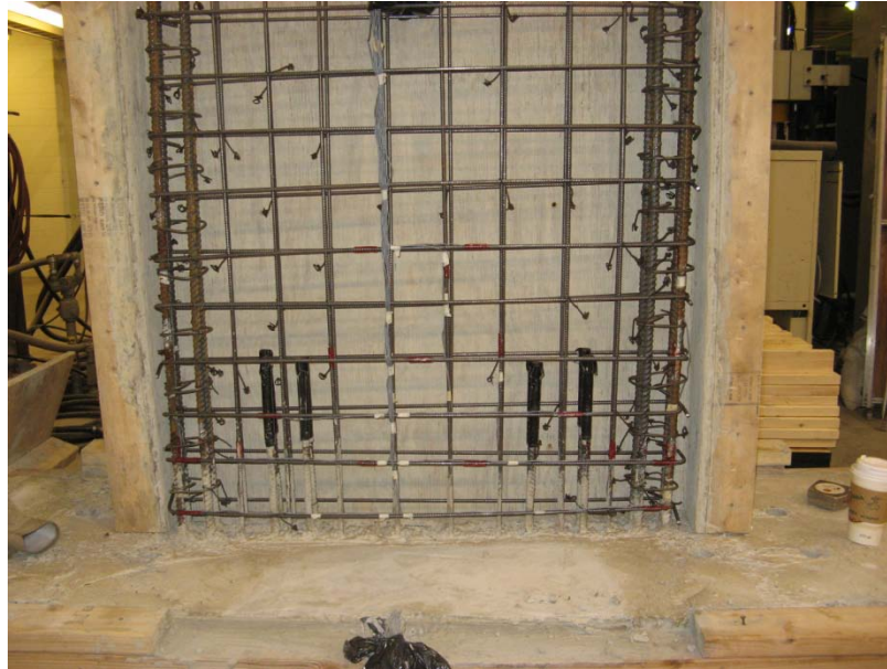
Fig. 3-7 Dowel Reinforcement in Specimen S5
