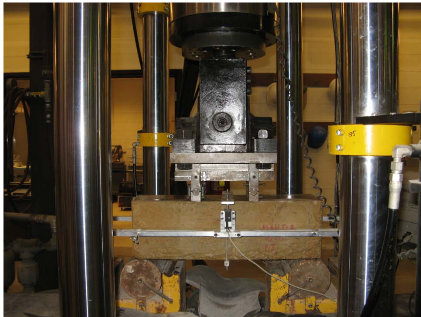
Fig. 3-17 ASTM 1609 Beam Test Set-Up
