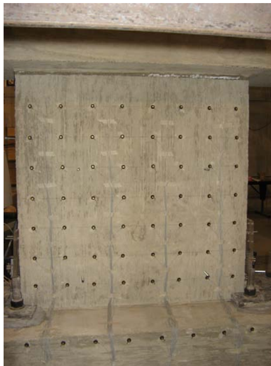
Fig. 3-32 Optotrak Instrumentation Scheme
