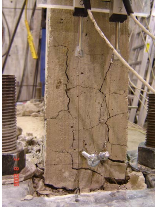
(c) close-up of wall boundary region at end of test (2.1% drift)
