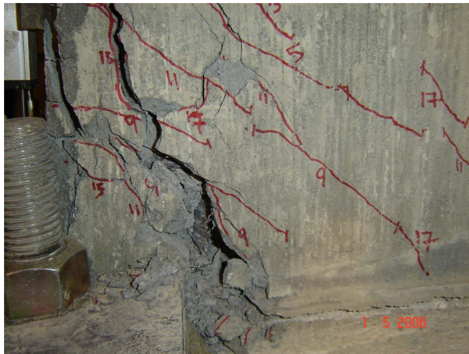
(d) close-up of boundary region after end of test (3.0% drift)
