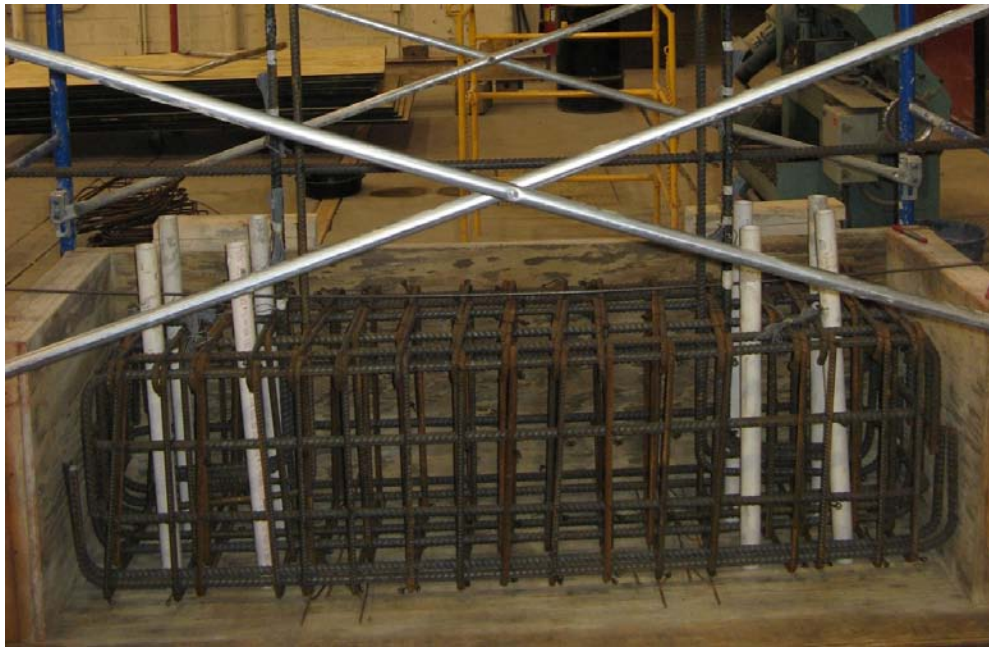
Fig. 3-21 Base Block inside Formwork (Specimen S4)
