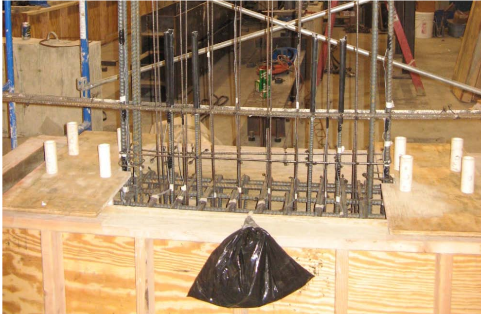
Fig. 3-22 Base Block Ready for Casting (Specimen S10)
