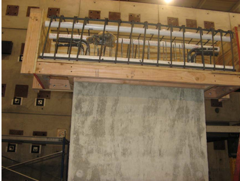
Fig. 3-26 View of Top Beam inside Formwork (Specimen S9)
