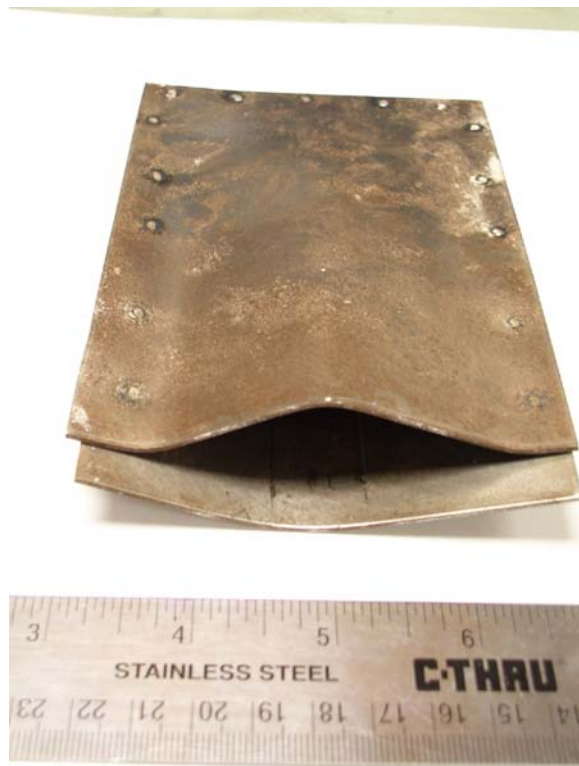
Figure 3.5 The steel jacket used to protect the Ti piece during heating and retain heat during rolling. Three sides of the bag were spot welded and the fourth side was opened so that the Ti-6Al-4V piece could be easily slid in.
