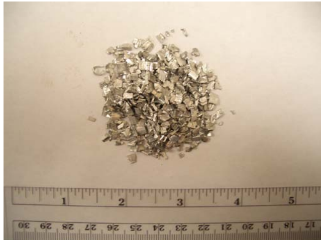
Figure 2.1 ZK60 chips provided by Thixomat.Inc..
