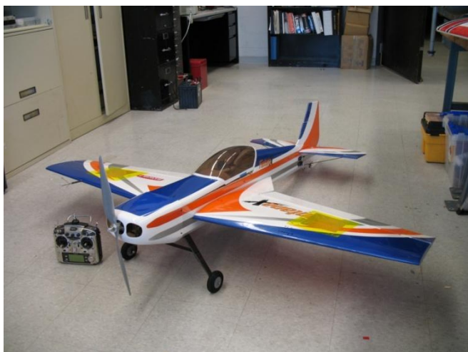
Figure 5: Funtana Test Aircraft (air data probe on right wing, chordwise pressure ports on left wing)
