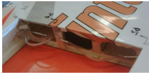
Figure 3: Wing Pressure Port Construction
