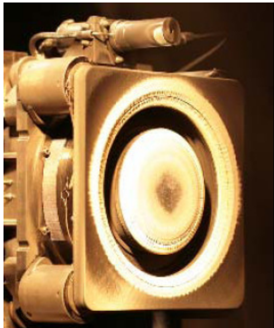
Figure 4 BPT-4000 showing 5800 hours of wear 1
