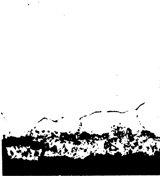
Fig. 17. Type 310 alloy. Heat X27258. 1900°F, 100 hours. Air velocity - 30 ft/min. 750X. Cross section, unetched.
