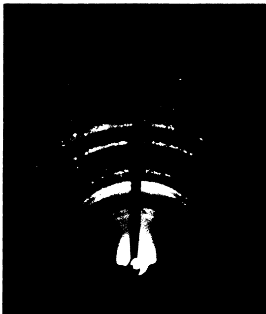
Fig. 5. Typical electron diffraction pattern of rhombohedral phase.
