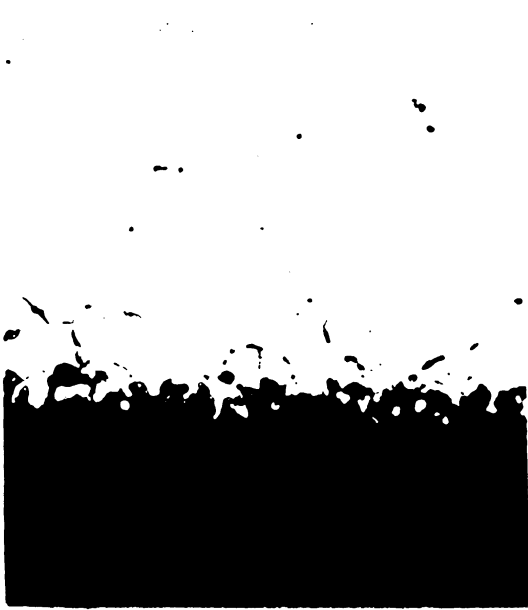
Fig. 11. Chromel ARM alloy. Heat A. 1900°F, 100 hours. Stress - 250 psi. 750X. Cross section, unetched.
