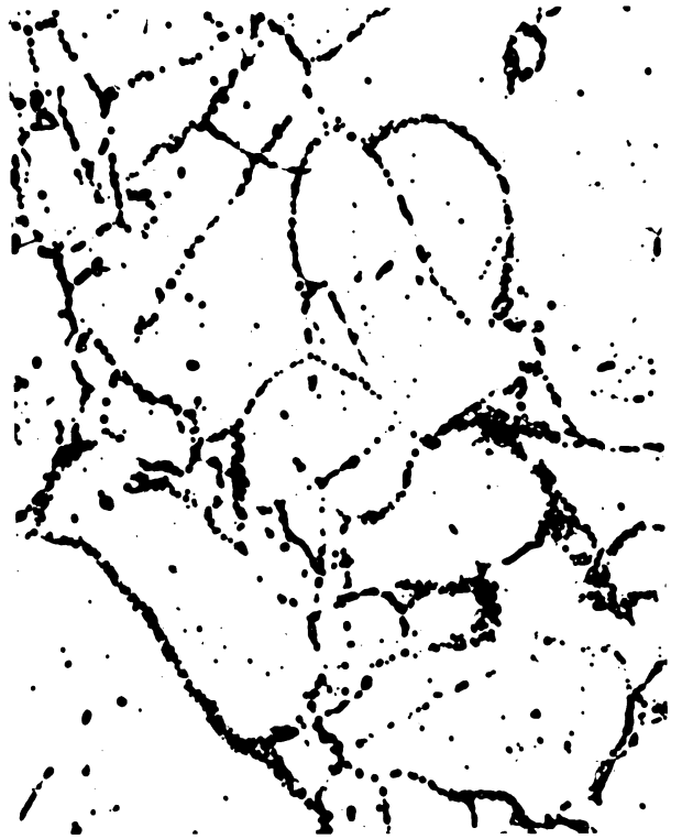
Fig. 10. Grain Boundary Network. Type 310 Alloy, Heat 64177. As Received. 1000x. Plane of Rolling. Etch: Electr. Chromic Acid.
