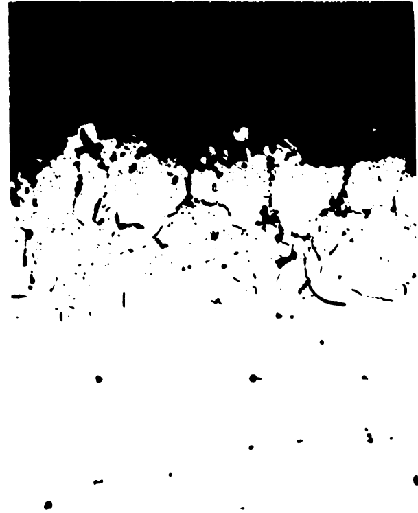
Fig. 106. Penetration and Precipitation. Type 310 Alloy, Heat X 11306. 2000°F and 10 hr. 750x. Cross Section. Unetched.
