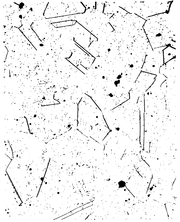
Fig. 6. Type 310 Alloy, Heat X 27258. As Received. 100x. Obl. Light. Plane of Rolling. Etch: Electr. 1:1:1 HCl, HNO 3 , H 2 O.
