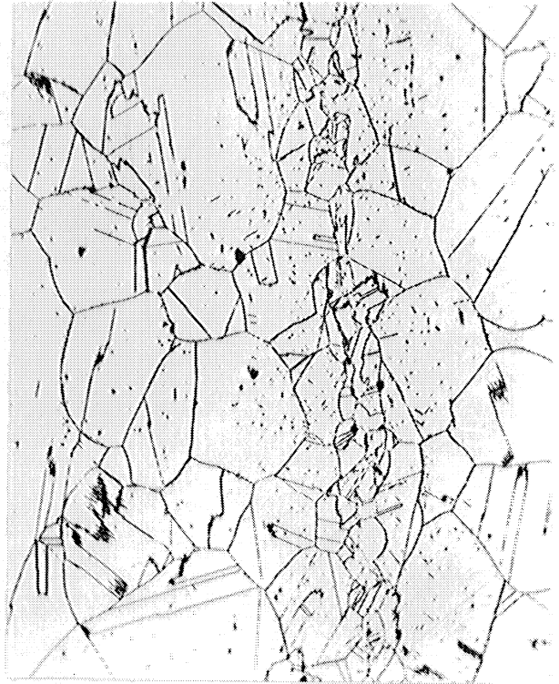
Fig. 118. Carbide Bands and Grain Refinement. Type 310 Alloy, Heat X 45558. 1600°F and 100 hr. 250x. Cross Section. Etch: Electr. Chromic Acid.
