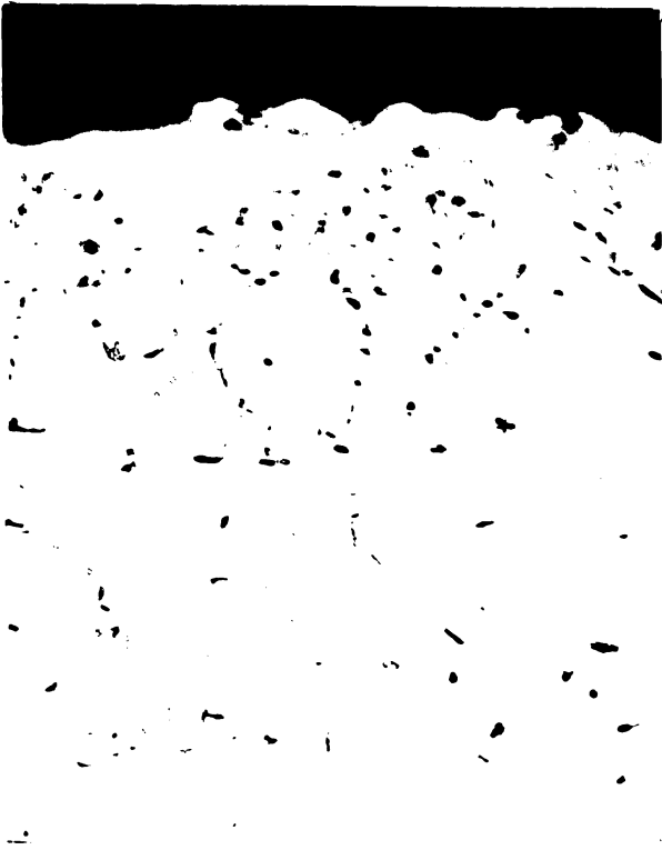
Fig. 103. Penetration and Precipitation. Type 310 Alloy, Heat X 11306. 1600°F and 100 hr. 750x. Cross Section. Unetched.
