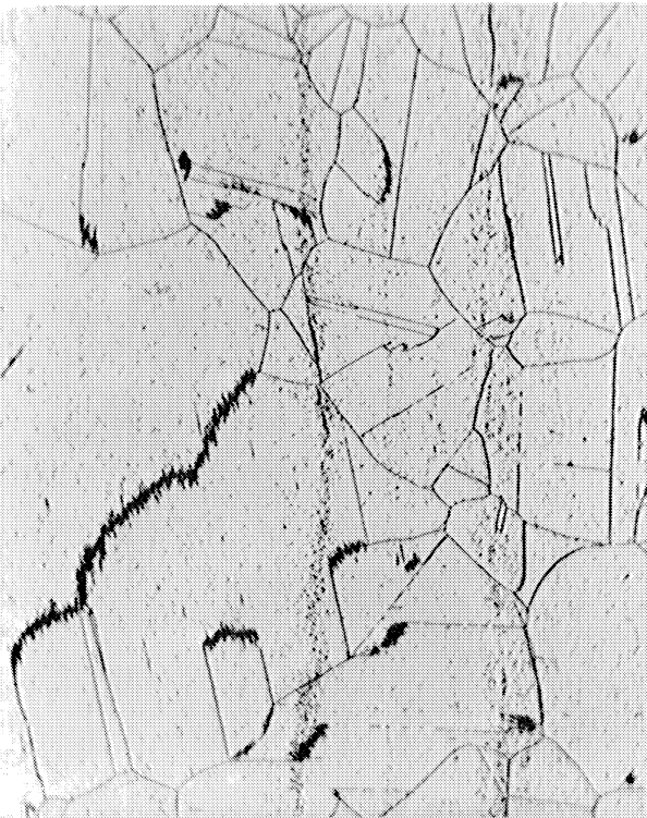
Fig. 117. Carbide Precipitation Bands. Type 310 Alloy, Heat X 45558. 1600°F and 10 hr. 250x. Cross Section. Etch: Electr. Chromic Acid.
