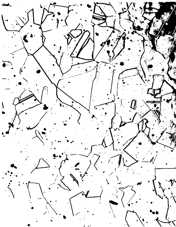
Fig. 7. Type 310 Alloy, Heat X 45558. As Received. 100x. Obl. Light. Plane of Rolling. Etch: Electr. 1:1:1 HCl, HNO 3 , H 2 O.
