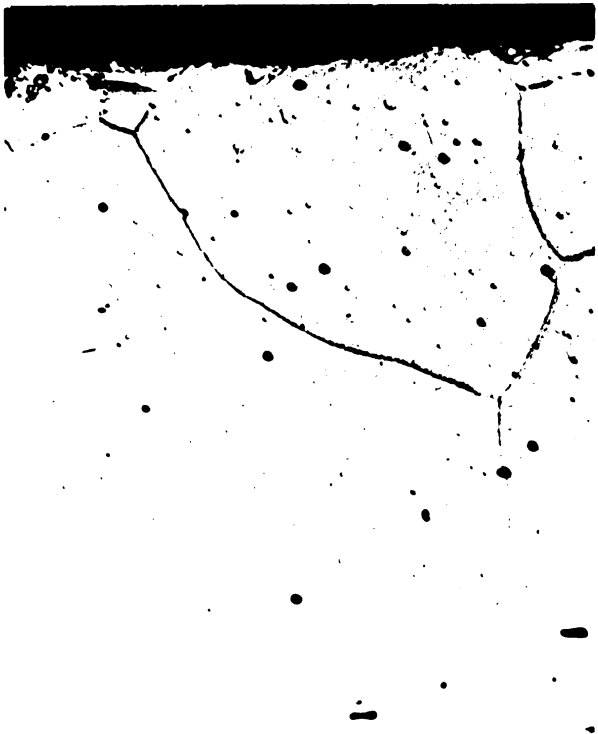
Fig. 101. Grain Boundaries before Testing. Type 310 Alloy, Heat 64270. As Received. 750x. Cross Section. Etch: Electr. Chromic Acid.
