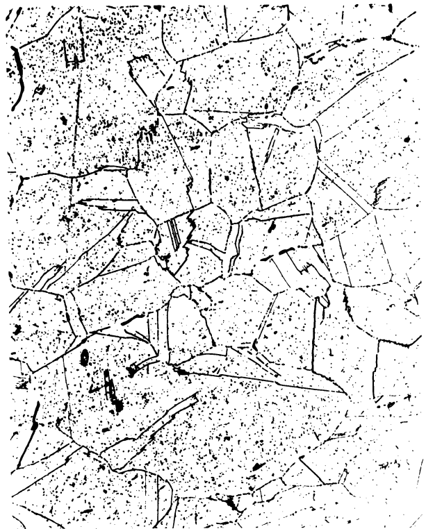
Fig. 112. Matrix and Boundary Precipitation. Type 310 Alloy, Heat X 11338. 1600°F and 100 hr. 250x. Cross Section. Etch: Electr. Chromic Acid.
