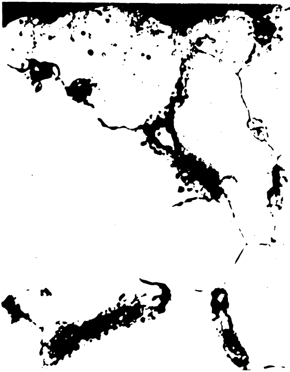
Fig. 99. Type V Penetration. Developed Web. Type 310 Alloy, Heat X 11338. 1900°F and 100 hr. 750x. Cross Section. Unetched.
