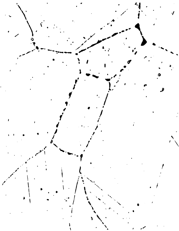
Fig. 111. Sigma Phase. Type 310 Alloy, Heat X 27258. 1600°F and 100 hr. 1000x. Cross Section. Etch: Murakami's Reagent.
