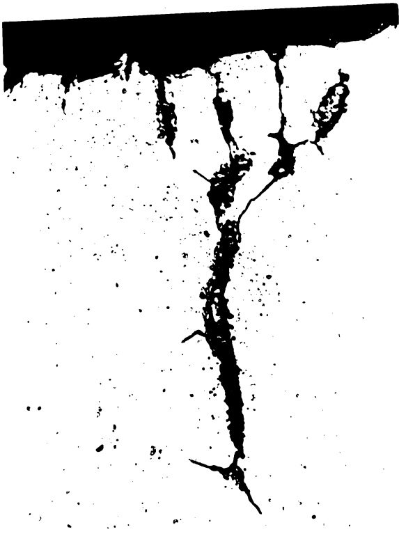
Fig. 107. Developed Web Penetration. Type 310 Alloy, Heat X 11338. 1900°F and 100 hr. 750x. Cross Section. Etch: Electr. Chromic Acid.
