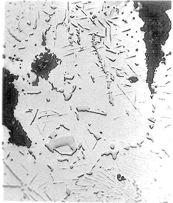
Fig. 11. Excess Constituent and Pre-rupture Fissures; Type 310 Alloy, Heat X46572, 1900°F, 100 Hours, Stress 1000 Psi, 750X; Cross Section, Unetched, Oblique Light.
