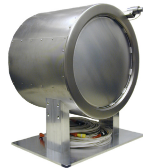
Figure 2. Laboratory model 4 (LM4) 40-cm NEXT ion thruster.
