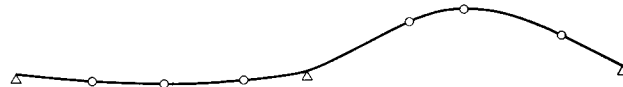
Fig. 13b First mode shape of mistuned two-span beam, for \overline{\Delta l} = 0.02 and \bar{c} = 281.8 , from measurements.
