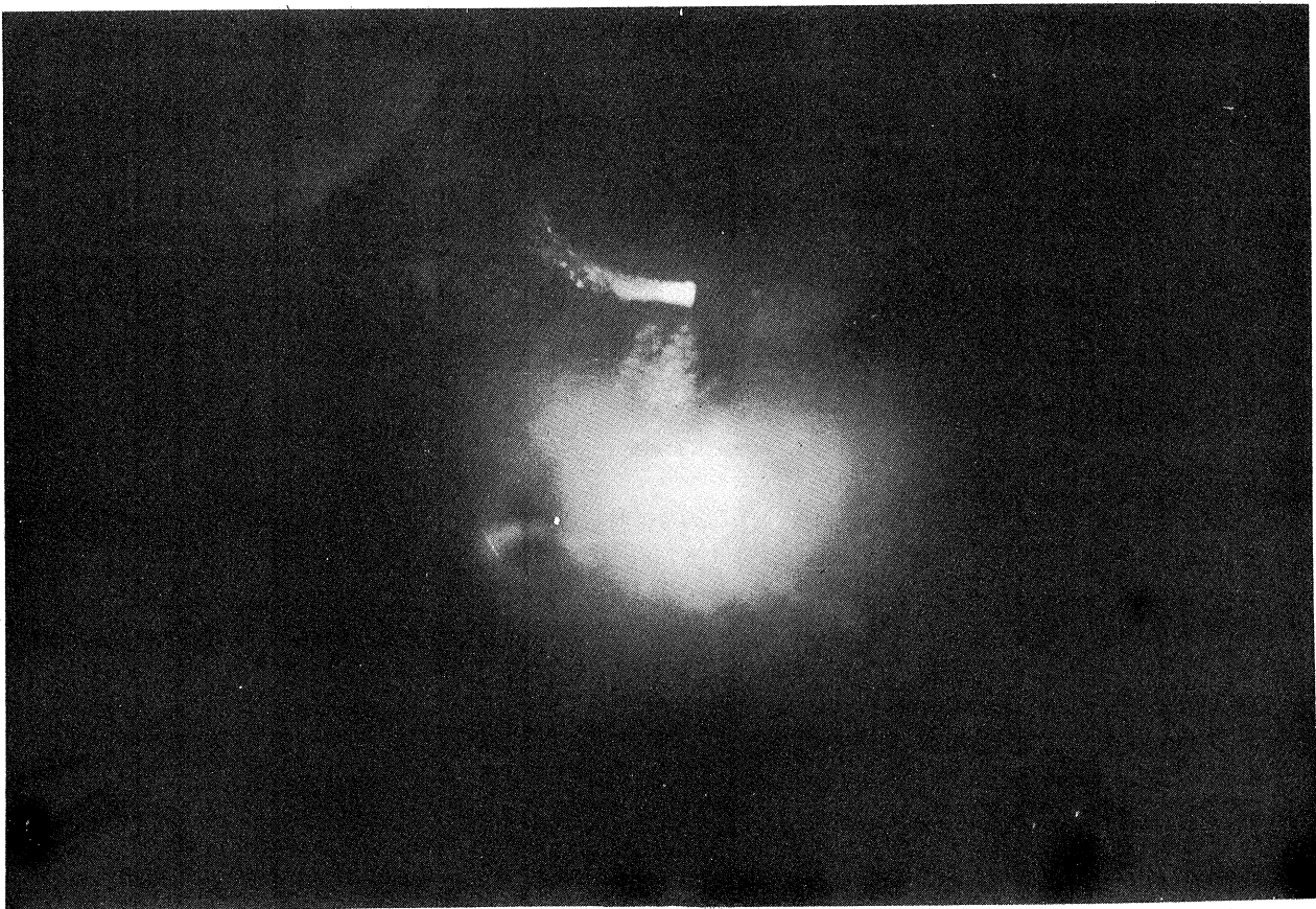
Fig. 13 "Total exposure" picture; Impulse potential - 6 kv Single "hot" electrode
