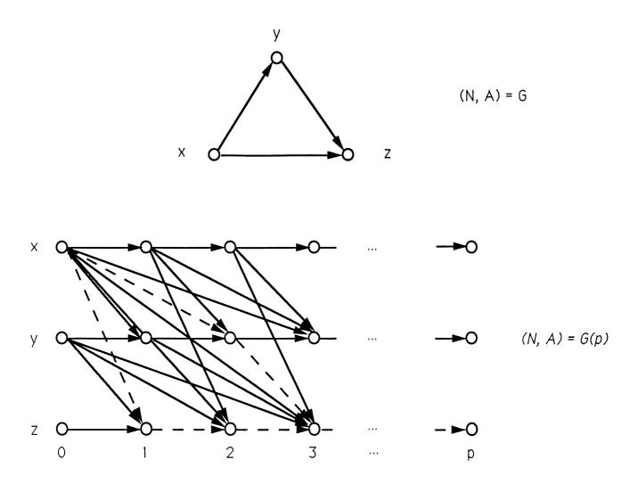
Figure 1 - Triangle network with two alternate routes
