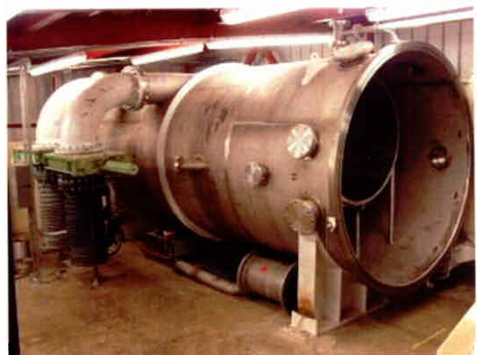
Figure 28. JPL liquid metal fed thruster test facility.
