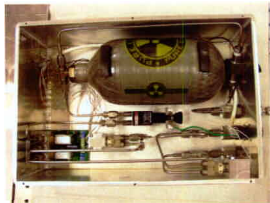
Figure 26. Bismuth tank pressurization system.
