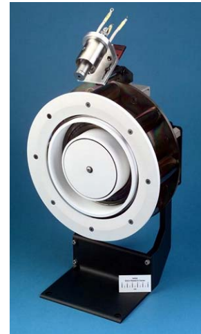
Figure 2. NASA-173Mv1 Hall Thruster
