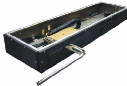
Figure 3. High-Speed Axial Reciprocating Probe System
