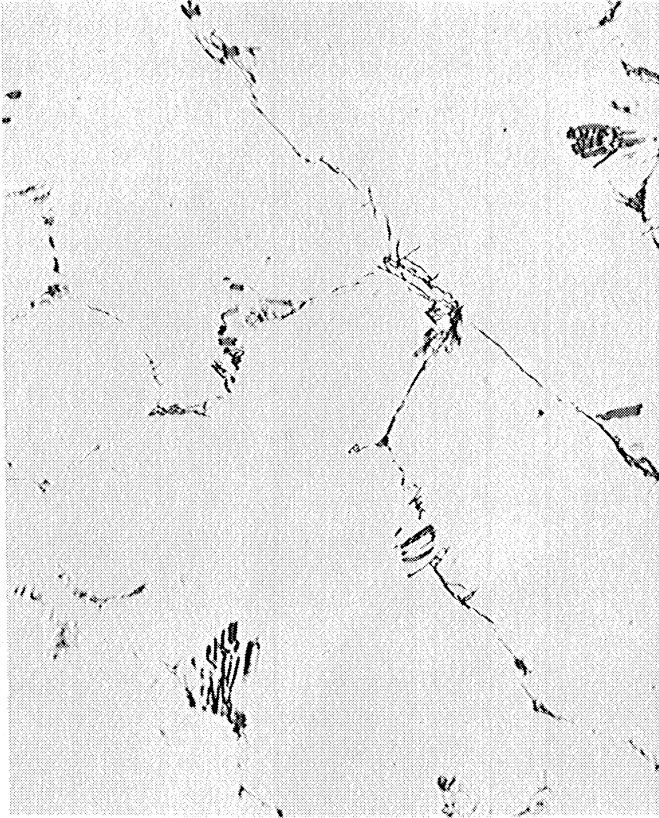
(a) Heat R105, containing 0.5% boron, shows a limited amount of grain boundary constituent.
