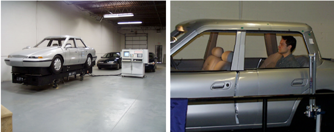
Figure 1. Reconfigurable vehicle mockup. PVM and control unit in UMTRI laboratory (left) and left side view (right).
