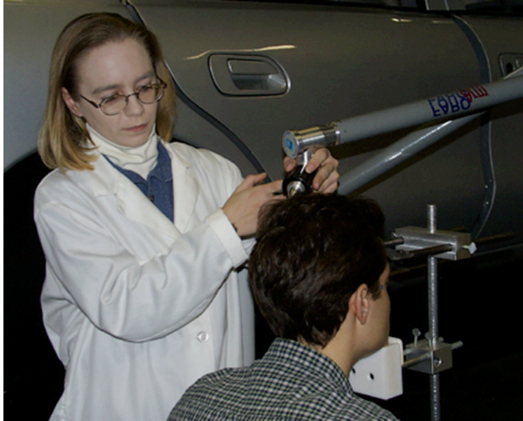
Figure 3. Head digitization with subject resting in stabilization fixture.
