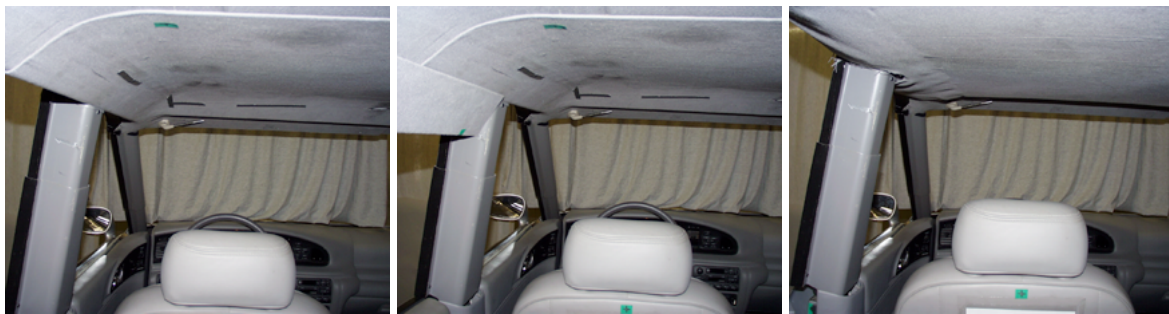
Figure 6. Three different roof contours. PVM shape (left), rail insert (middle), roof insert (right).
