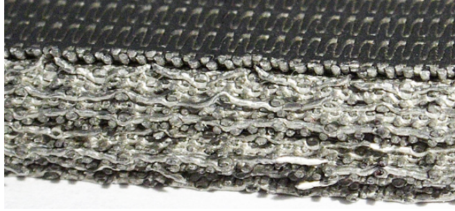
Figure 5.2: Rigimesh cross section after bending fracture.
