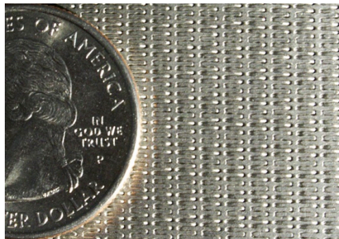
Figure 5.1: Surface features of the Rigimesh material used in SSME.
