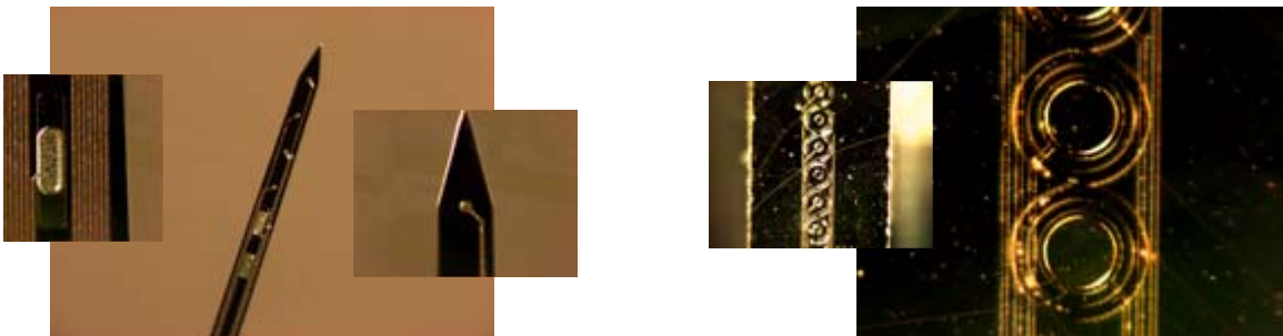
Figure 4.7: Micrographs of chemical probes. These are micrographs of the probes fabricated for this project. The probe in the picture on the left shows a Michigan style neural probe with integrated reference and counter electrodes. The probe on the right is one of the test structure probes with SU-8 rings for site specific coatings. ©2005 IEEE. Used with permission from [Franklin05].
