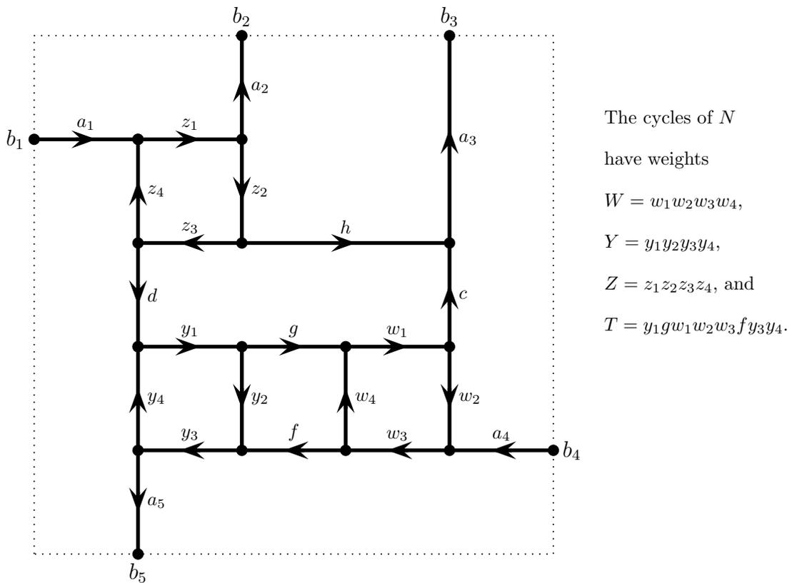
Figure 3.1: A planar circular network  $N$  with boundary vertices  $b_1, b_2, b_3, b_4, b_5$ . Edges are labeled by their weights.
