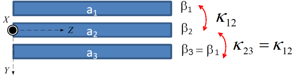
Figure 4.7: Three coupled channel waveguides. Waveguides 1 and 3 are identical and equidistant from waveguide 2.
