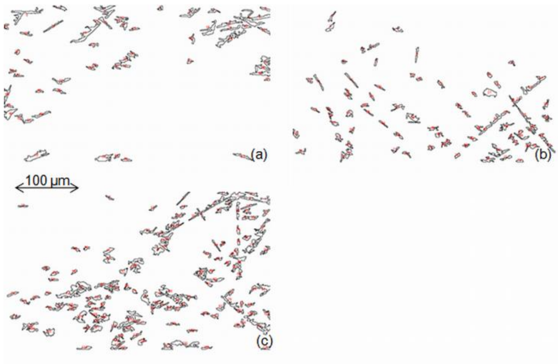
Figure 3.7. Representative images produced by thresholding algorithm that are used to analyze the number of cavities available for nucleation in (a) baseline, (b) Surface #1, and (c) Surface #4.
