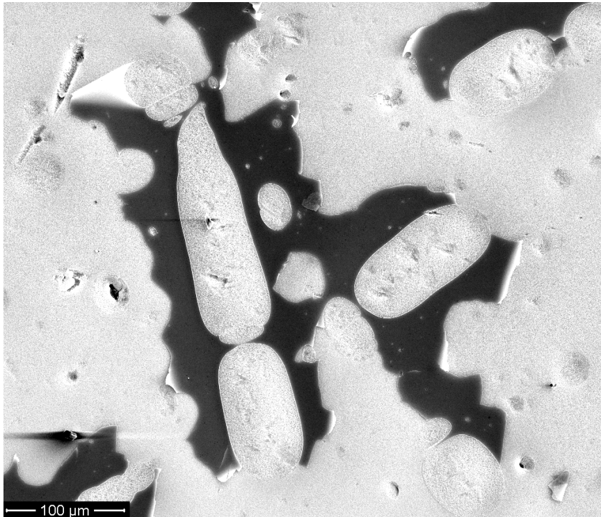
Figure A3.4. Plan-view SEM image of GaSb irradiated with 1 MeV Au + to an ion fluence of 6 \times 10^{14} ions/cm 2 .
