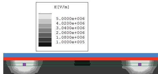
Fig. 4.7 E-M Simulations of a Low-Density NW-TFT
